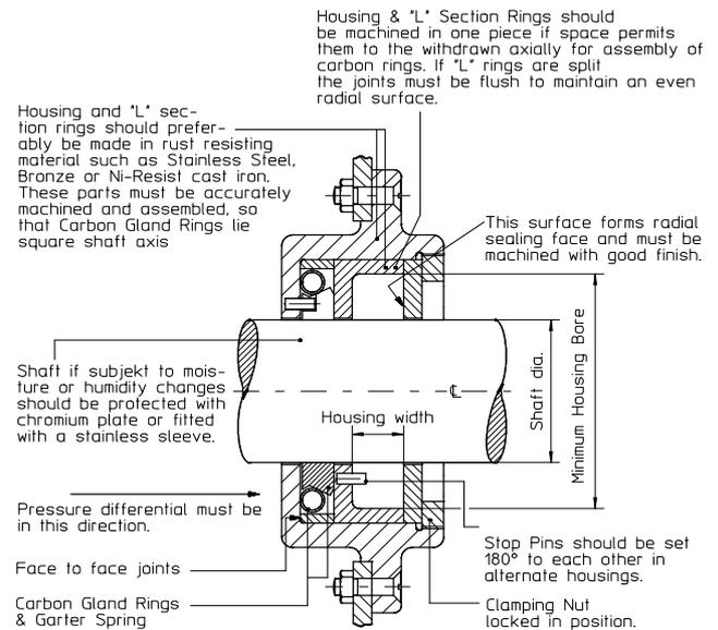
Sketch 4 Bevel Section Carbon Gland Rings in 'L' Section Housing
