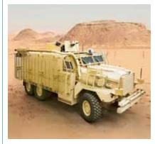
A new ceramic protection system developed by the Defence Science and Technology Laboratory and NP Aerospace, is being used to protect troops and military vehicles from the threat of improvised explosive devices and machine-gun fire.
