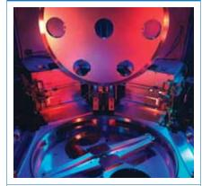
Morgan AM&T's material expertise and custom process solutions is helping semiconductor device manufacturers to reduce the line width by 50% (45nm to 22nm in 2016) with ultra-pure, precision-machined graphite components used in the manufacturing processes.
