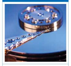
Morgan Technical Ceramics makes piezoceramic actuator plates for disk drive storage in devices from HD-TVs to PCs. Ceramic enables the head to be positioned with greater accuracy allowing for higher capacity without increasing disk size.
